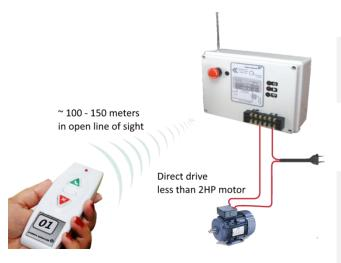
Wiring diagram to connect the motor/pump directly to the main AC supply.
